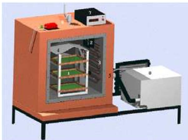
**Figure 2: Pictorial View of the Lab Scale CA Chamber (Mahajan, 2001) (1 – Fruit Tray, 2 – Evaporator Fan, 3 – Evaporator Coil, 4 – Protection Cover, 5 – Outlet Valve, 6 – LN<sub>2</sub> Inlet, 7 – Temperature Controller and 8 – Refrigeration System)**
