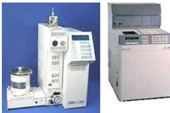
**Figure 5: Pictorial View of the Headspace Sampler and GC – FID Used for Aroma Analysis**
